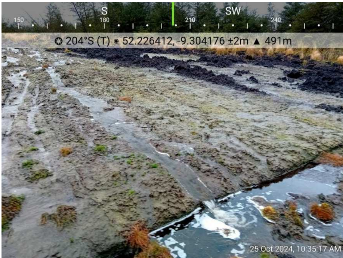
Figure 4-8: Potential basal peat shear plane with flow paths, and contour parallel drain visible in foreground.
