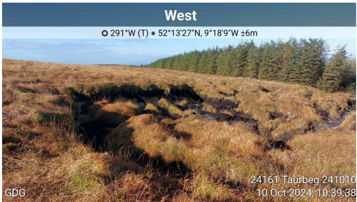
Figure 4-6: Arcuate, concentric tension cracks at the head scarp of ME-B.
